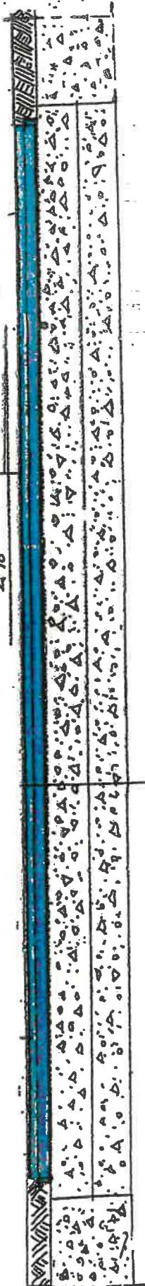
WARSTWA ŚCIERKOWA Z MIESZANEM MINERALNO-ASFALTOWYM GRUB. 16 CM
